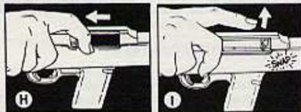
Pull charging handle all the way back. Let it snap forward freely.
